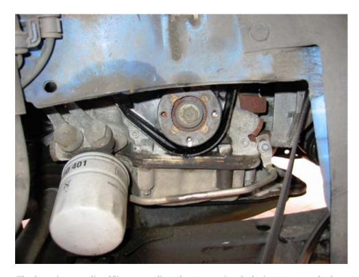
Check tensioner reading. If incorrect adjust, then turn engine clockwise two turns, check again, if incorrect keep adjusting and returning till it is correct.
